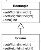
The clientMethod method makes an assumption that is true for Rectangle: setting the width respectively height has no effect on the other attribute. This assumption does not hold for Square.
