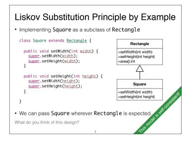
With this overriding of setHeight and setWidth – to set both dimensions to the same value – instances of Square remain mathematically valid squares. A square does comply to the mathematical properties of a rectangle: A square has four edges and only right angles and is therefore a rectangle.
