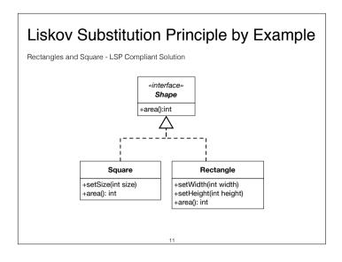
To get a LSP compliant solution, we make Rectangle and Square siblings. We introduce the interface Shape to bundle common methods.
