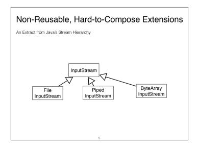
Consider an extract from java.io package that consists of classes for reading from a source. Streams abstract from concrete data sources and sinks:
