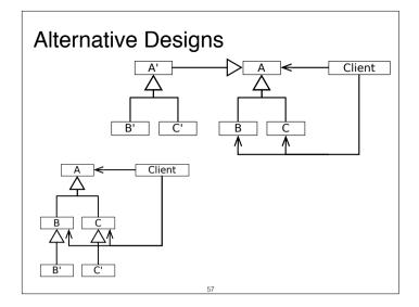
There are two possibilities ((I) creating a parallel hierarchy or (II) creating additional subclasses of B and C) to add an optional feature to A incrementally without affecting clients in a single inheritance setting.
