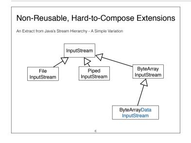
Need a variation of ByteArrayInputStream capable of reading whole sentences and not just single bytes.
