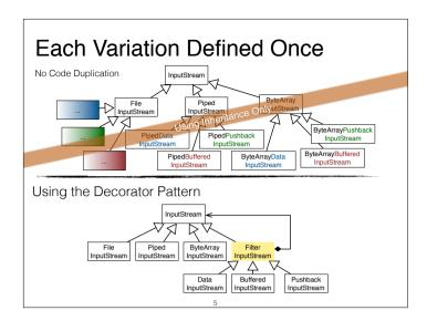
Decorator-based designs share the desired properties of corresponding designs based on inheritance only that **variations are well modularized**. We define one class per variation of base and decorative functionality.
